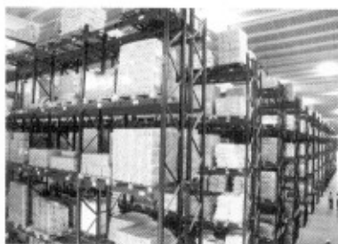
Selective Pallet Racking
